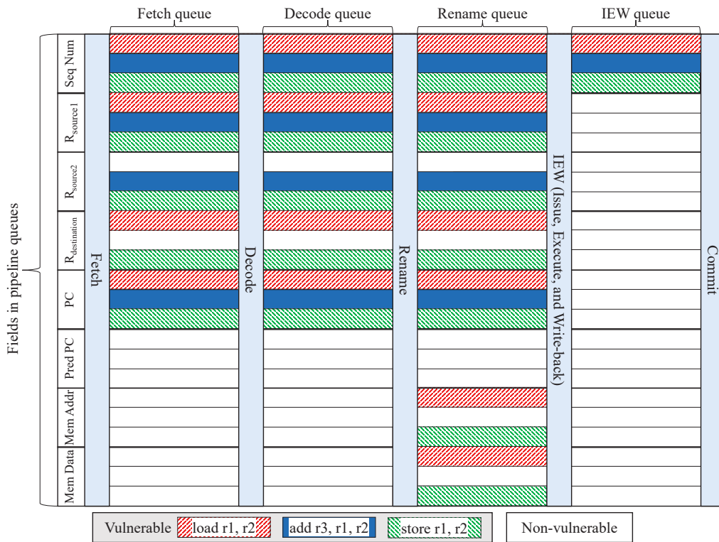
Figure 3.1: Fine-grained vulnerability tracking for pipeline queues for simple instructions such as load (red), add (blue), and store (green)
